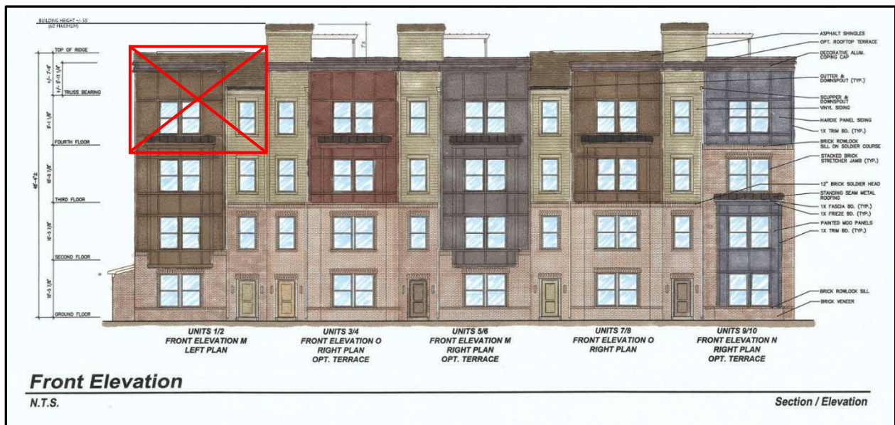
Figure 4. Illustrative Example showing the front elevation of a row of the Townhomes. The red box indicates the portion of the fourth floor to be removed, creating a single 3-story unit on the end of each row of the Townhomes.
